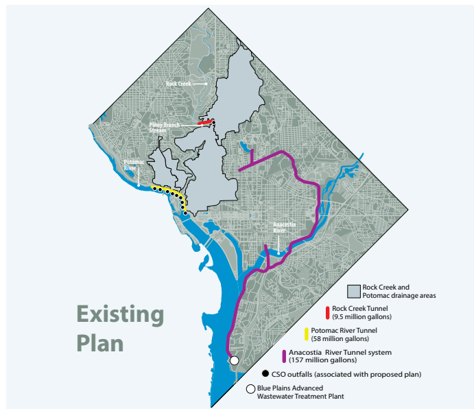
Figure 21: Original Clean Rivers Project Plan showing three major tunnel projects (Image credit: DC Water, 2015, source: https://www.dwater.com/education/gi-images/maps_existing_updated.pdf )
